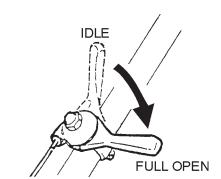
Figure 10. Throttle Lever (Full Open)
